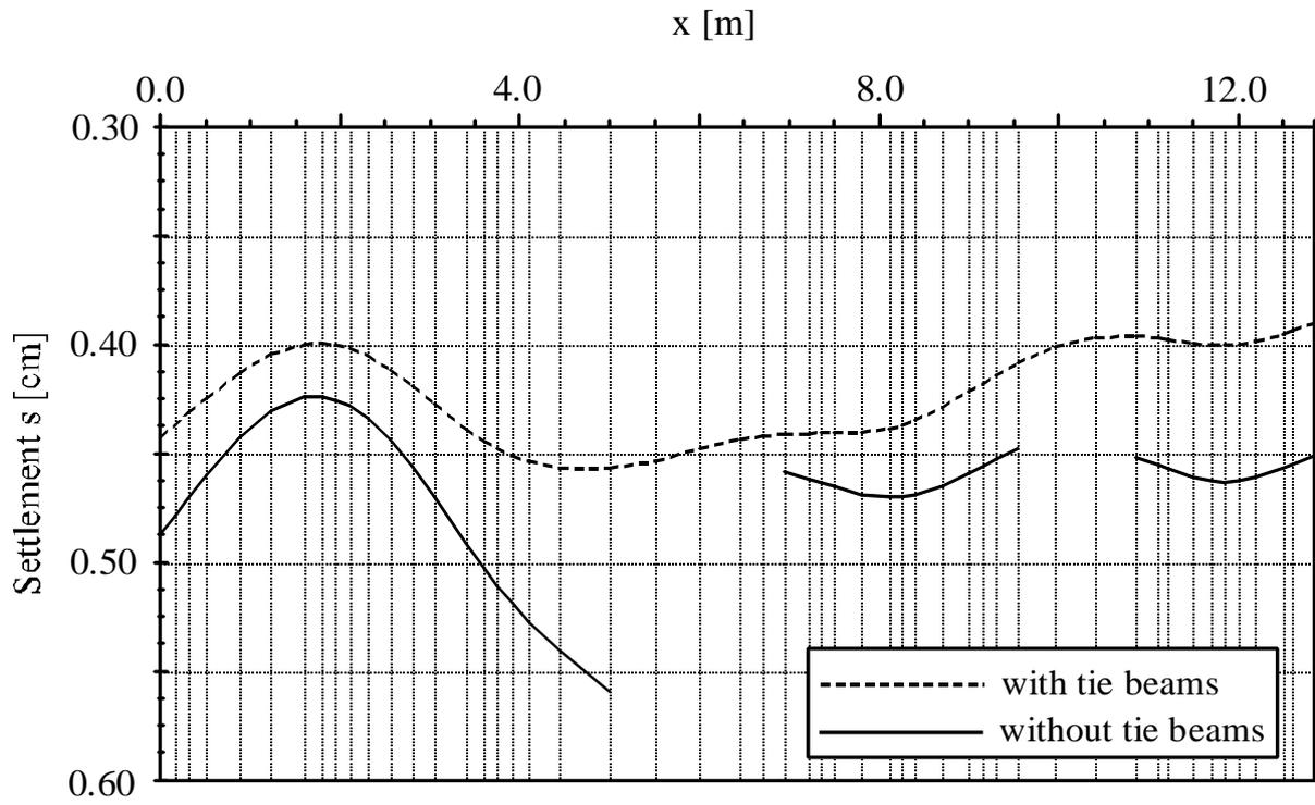
Figure 100 Settlement  $s$  [cm] at section 2-2
