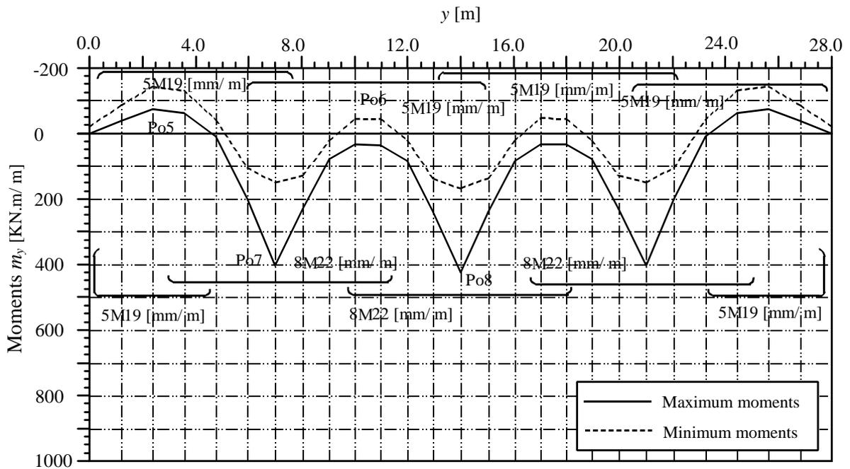
Figure 70 Extreme values of moments  $m_y$  [ $\text{kN.m/m}$ ] in field strip (2)
