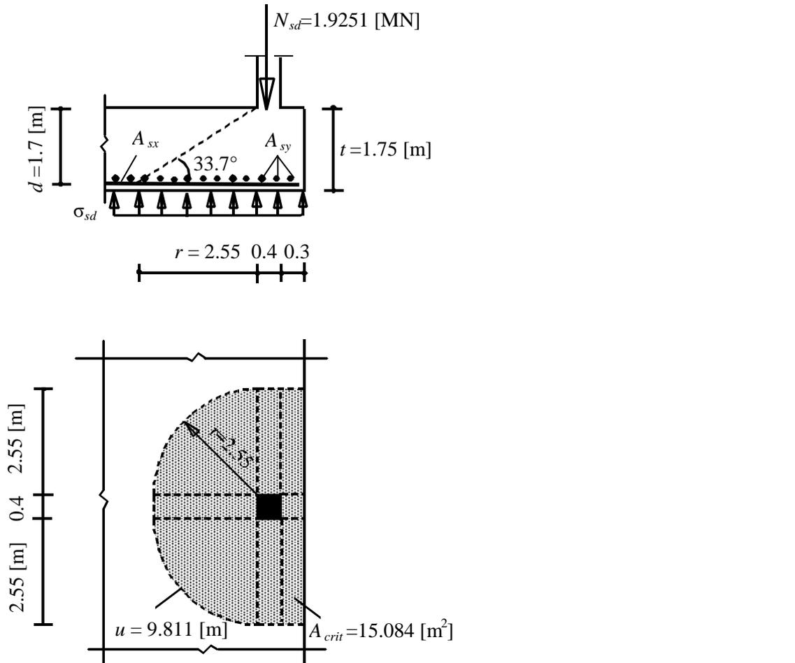
Figure 31 Critical section for punching shear according to EC 2
