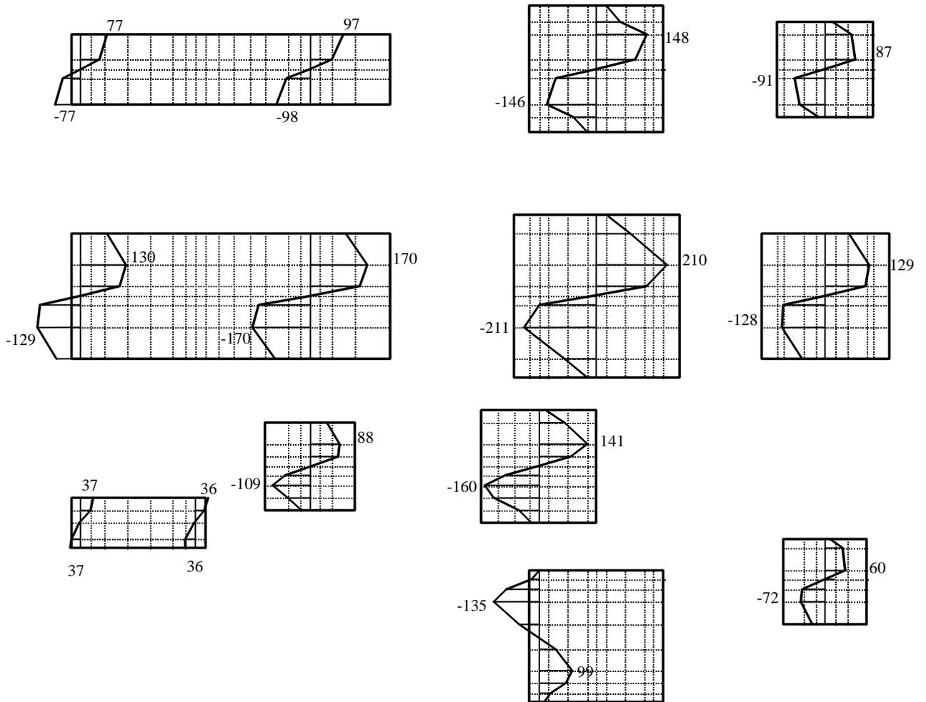
Figure 93 Shearing force  $Q_y$  [kN/ m] at critical sections on the footings
