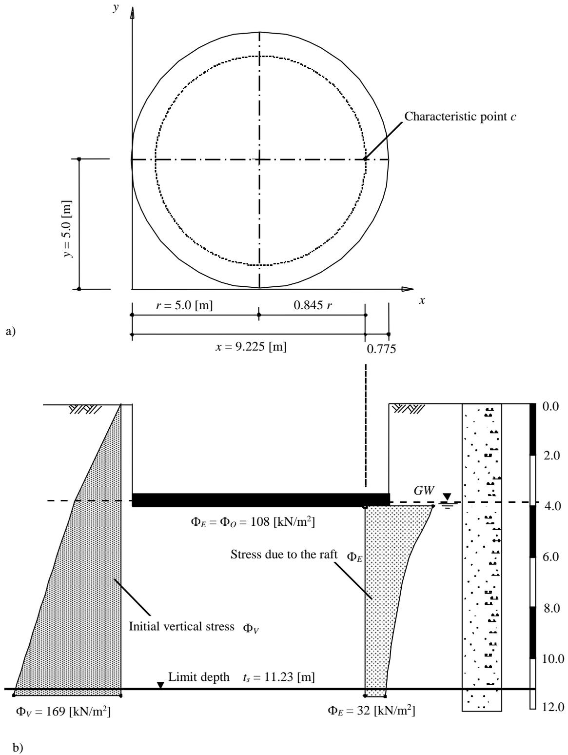
Figure 36 a) Position of characteristic point *c*
