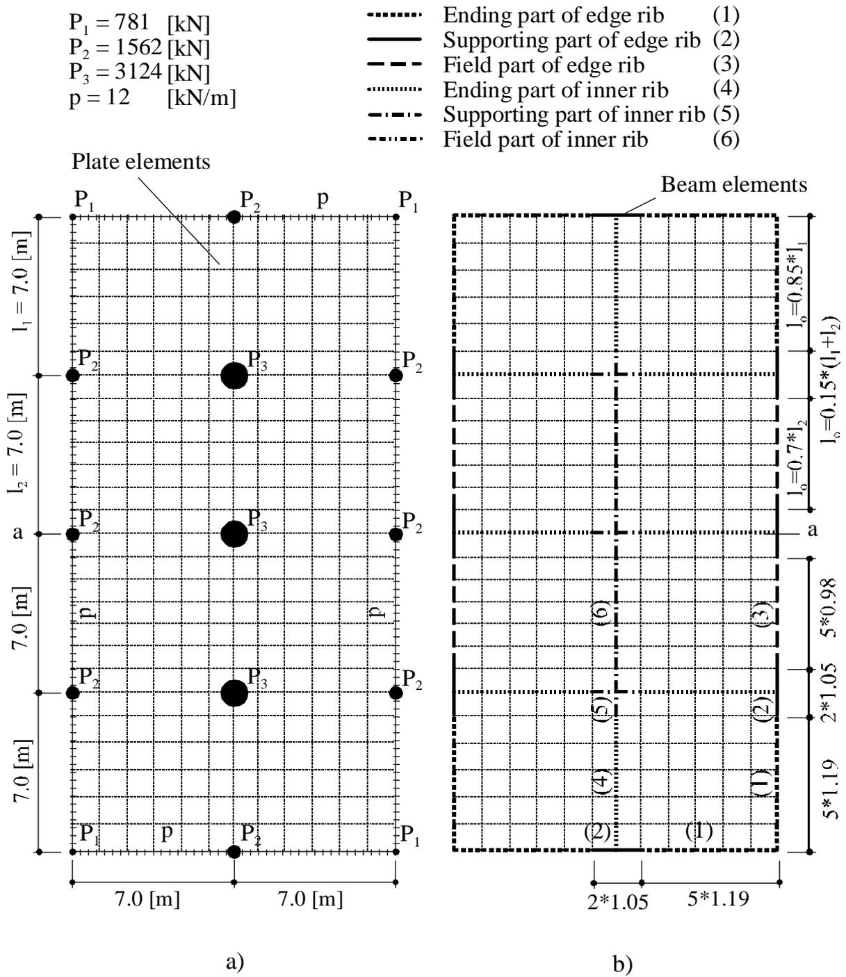
Figure 51 a) Flat raft with loads, dimensions and FE-Net
