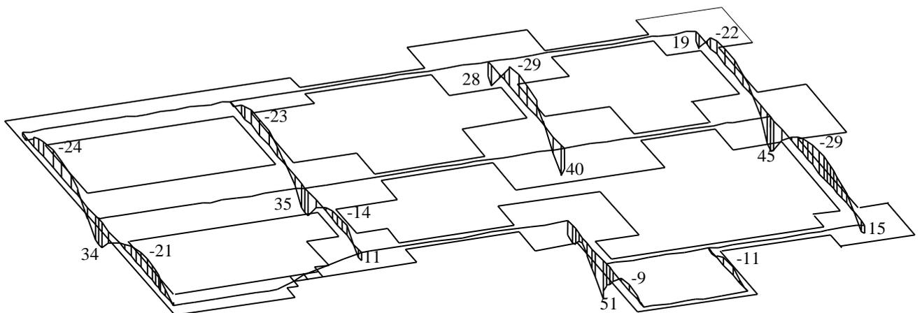
Figure 98 Moment  $M_b$  [kN.m] in girders at transversal direction
