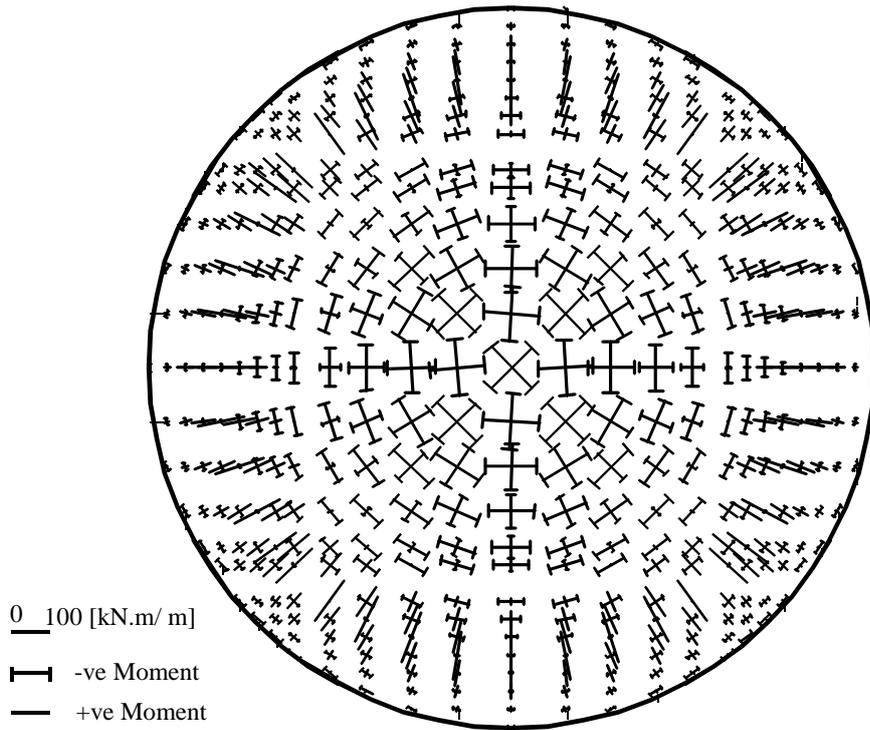
Figure 45 Vectors of principal moments  $h_{m1}$  and  $h_{m2}$  [kN.m/ m] of the raft without effect of the wall
