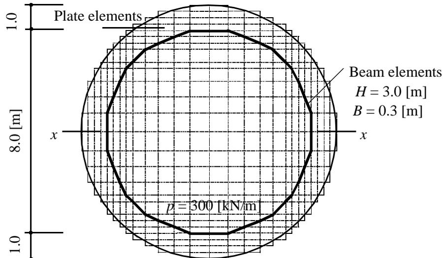
Figure 35 Rectangular finite element mesh
