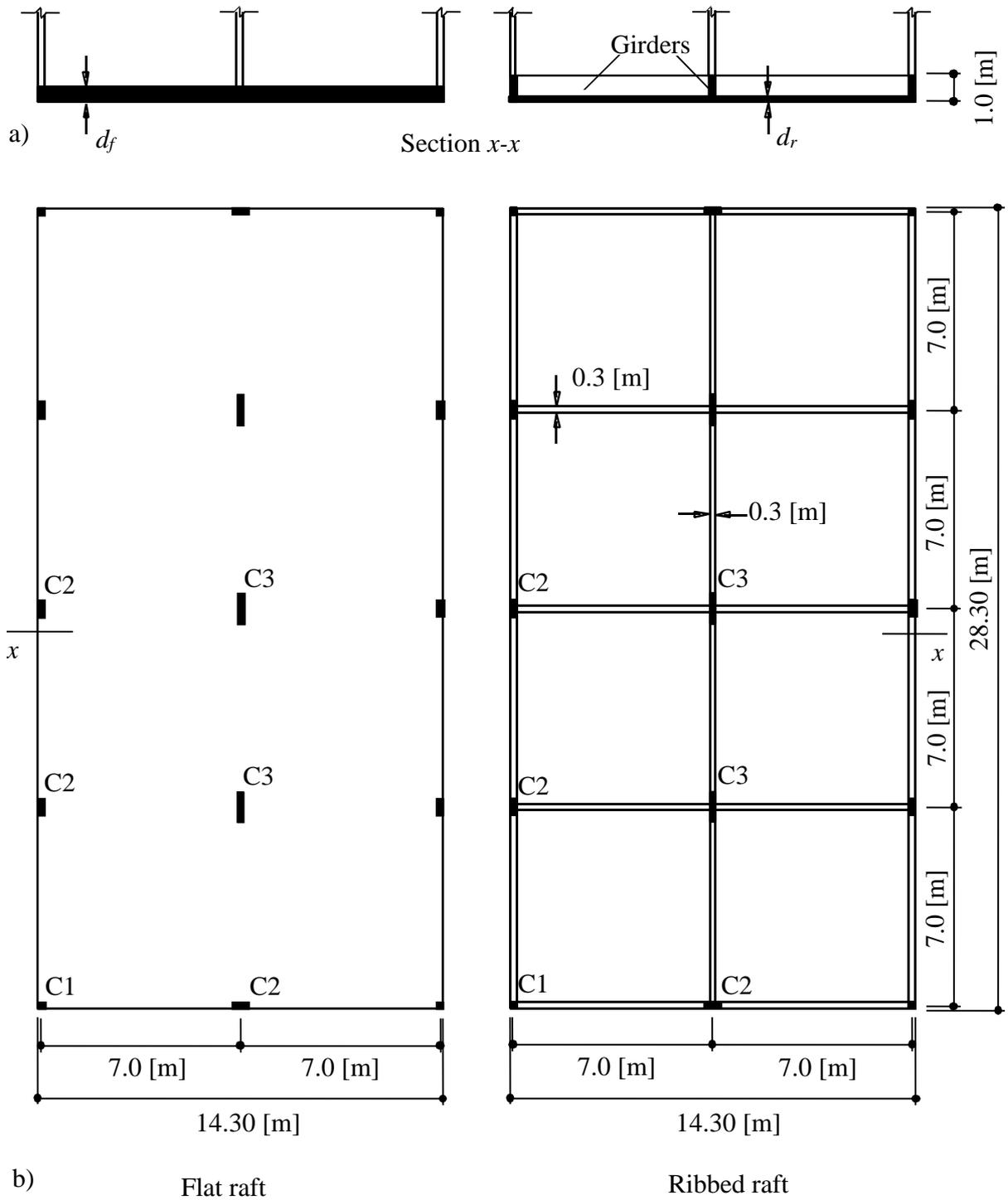
Figure 49 a) Plan of rafts and dimensions
