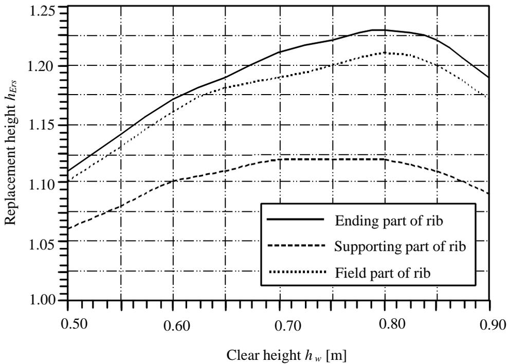
Figure 57 Replacement height  $h_{Ers}$  for inner ribs
