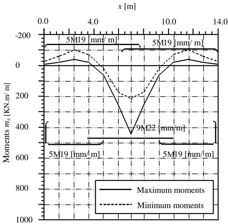
Figure 68 Extreme values of moments  $m_x$  [kN.m/ m] in field strip (IV)
