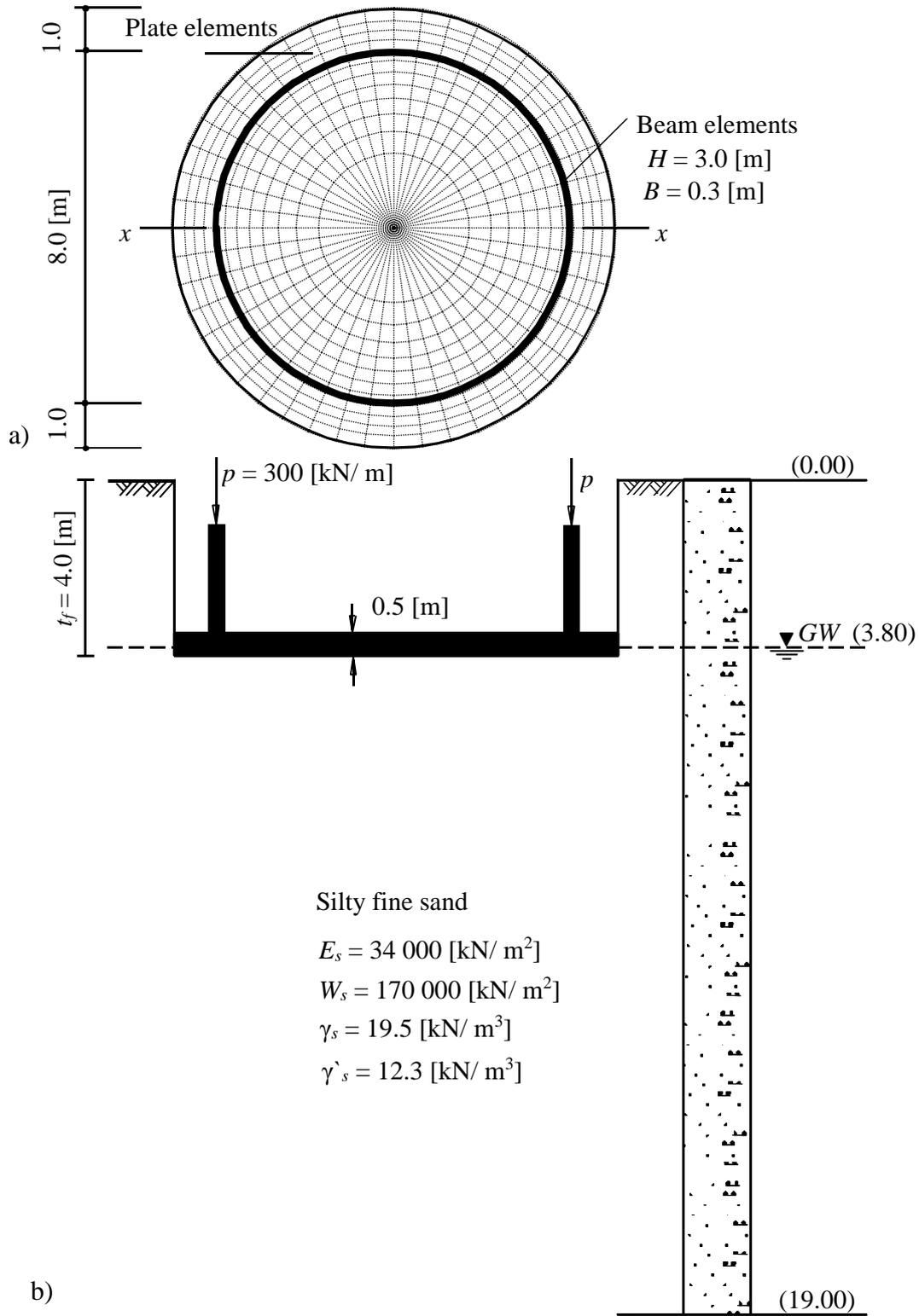
Figure 34 a) Plan of the raft with wall load, dimensions and mesh
