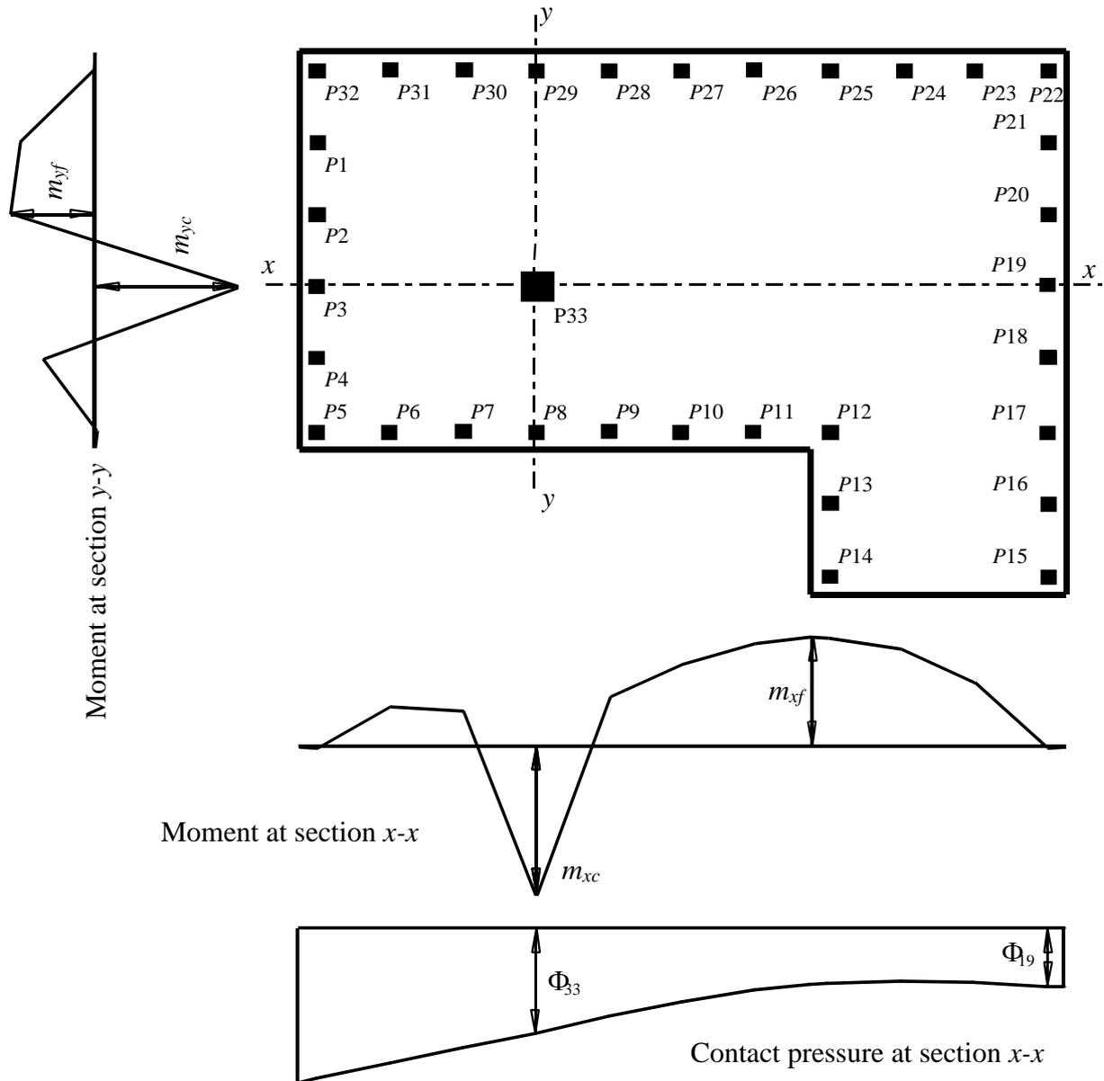
Figure 27 Definition of critical sections in  $x$ - and  $y$ -directions
