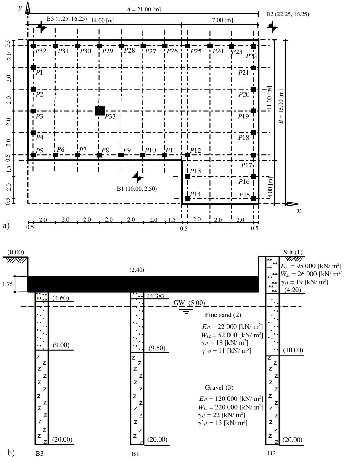
Figure 24 a) Plan of the raft with column loads, dimensions and mesh
