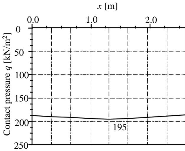
Figure 14 Contact pressure  $q$  [kN/ m<sup>2</sup>] at section I-I
