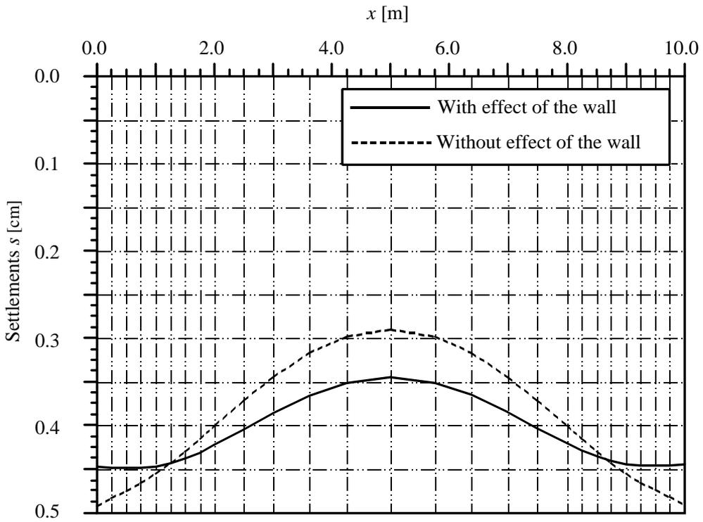
Figure 39 Settlements  $s$  [cm] at section  $x-x$
