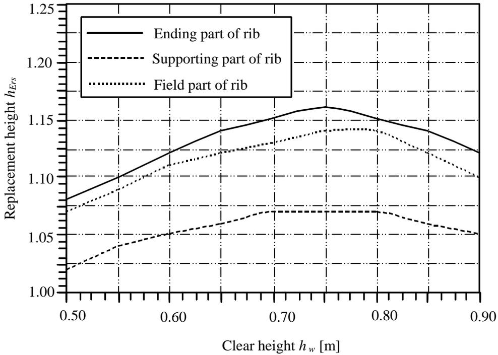
Figure 56 Replacement height  $h_{Ers}$  for edge ribs
