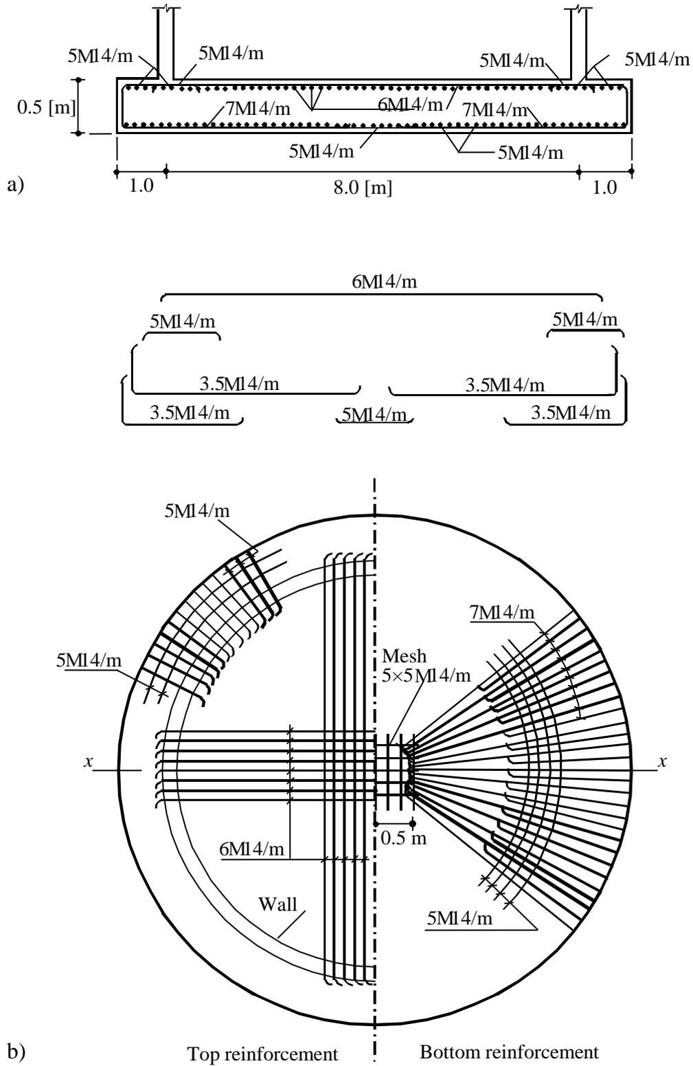
Figure 48 a) Section *x-x* through the raft with reinforcement
