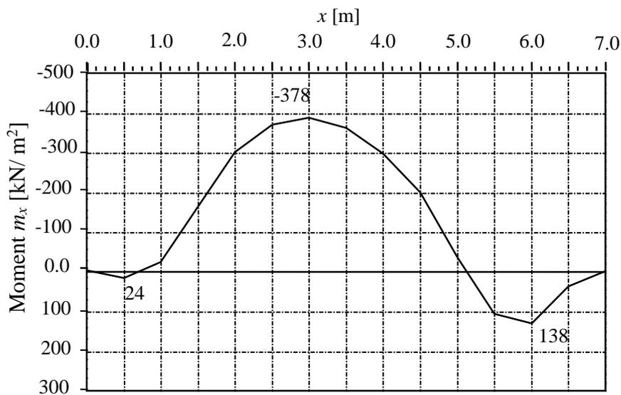
Figure 83 Moment  $m_x$  [kN.m/ m] at section *I-I*
