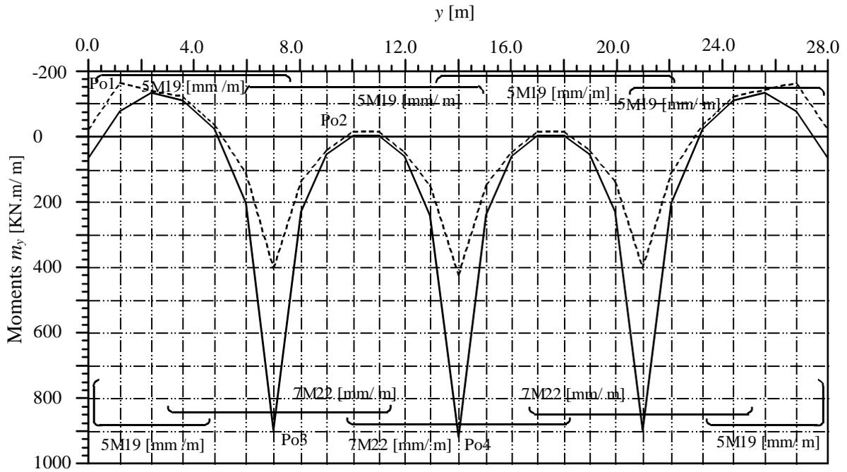
Figure 69 Extreme values of moments  $m_y$  [ $\text{kN.m/m}$ ] in column strip (3)
