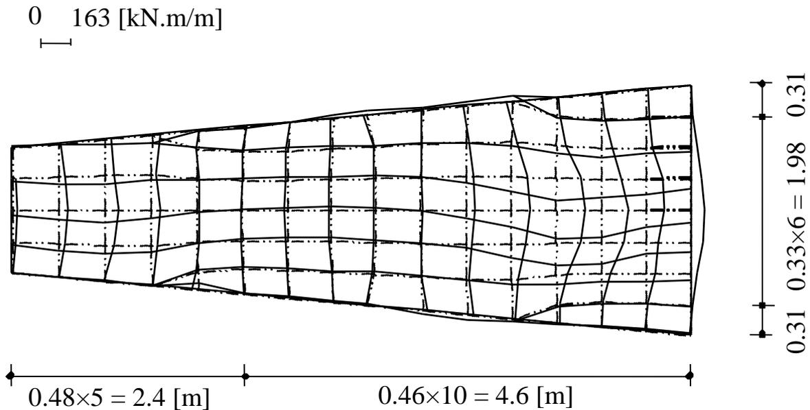
Figure 84      Distribution of the moment  $m_y$  [kN.m/ m] in the plan
