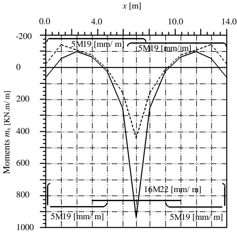
Figure 67 Extreme values of moments  $m_x$  [kN.m/ m] in column strip (III)
