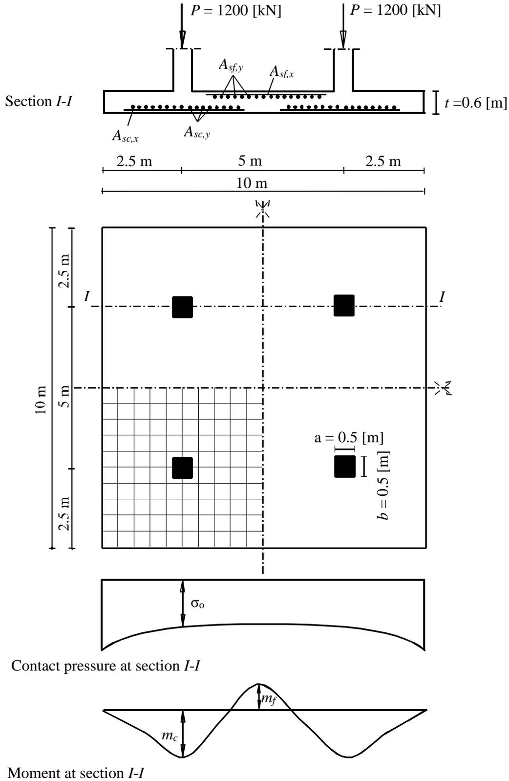
Figure 21 Raft dimensions with mesh and loads
