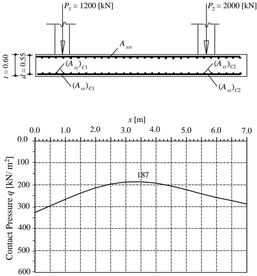
Figure 82 Contact pressure  $q$  [kN/ m<sup>2</sup>] at section *I-I*
