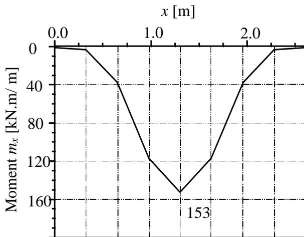
Figure 15 Moment  $m_x$  [kN.m/ m] at section I-I
