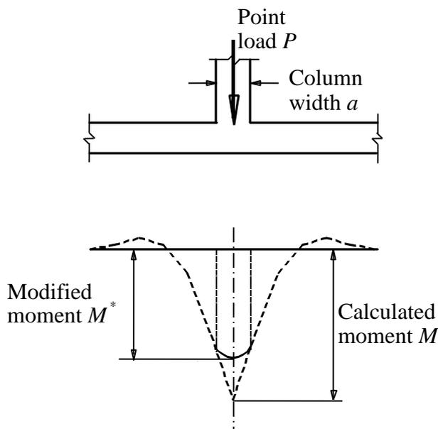
Figure 71 Modified moment under the column
