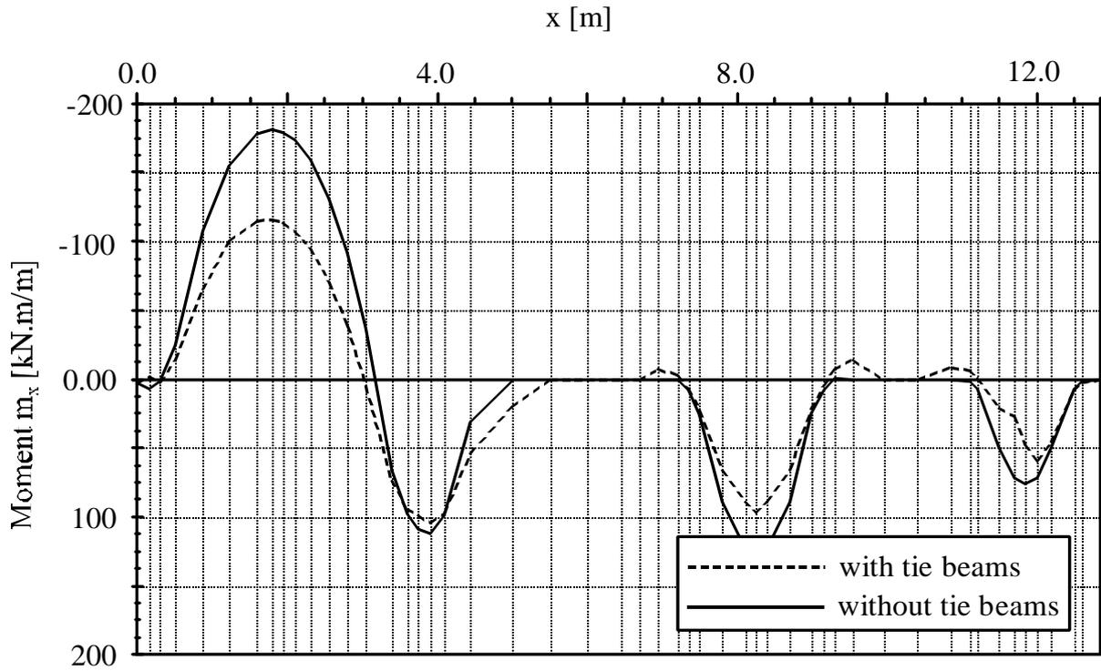
Figure 101 Moment  $m_x$  [kN.m/ m] at section 2-2
