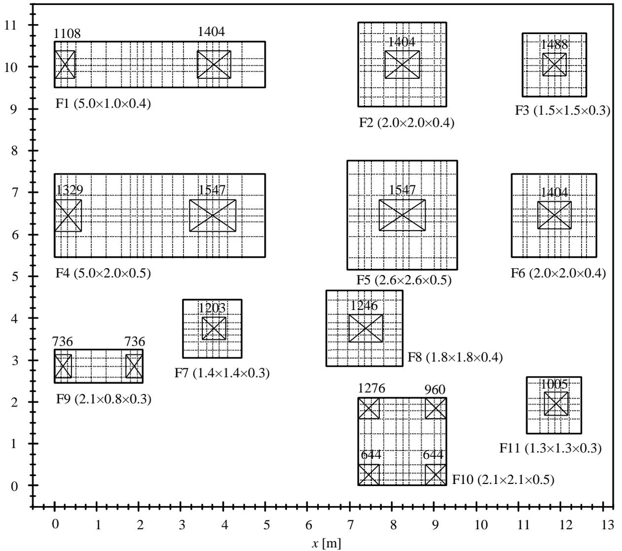
Figure 88 FE-Net of footings without tie beams, loads [kN/ m<sup>2</sup>] and footing dimensions [m]
