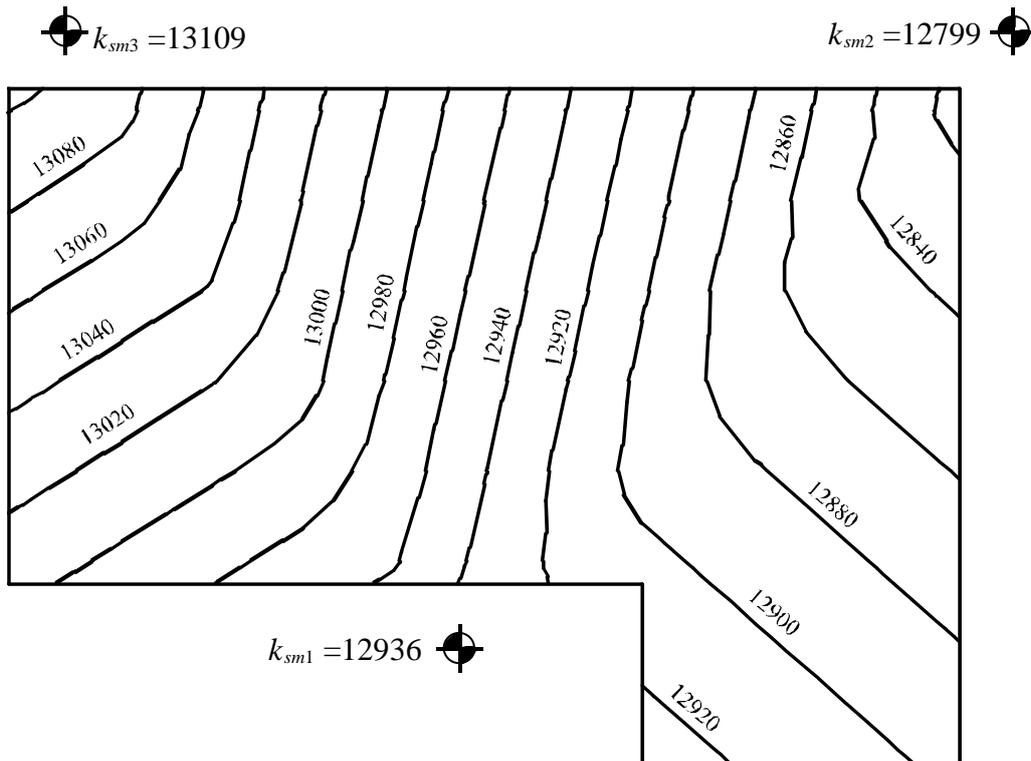
Figure 26 Contour lines for variable modulus of subgrade reaction  $k_s$  [ $\text{kN}/ \text{m}^3$ ]
