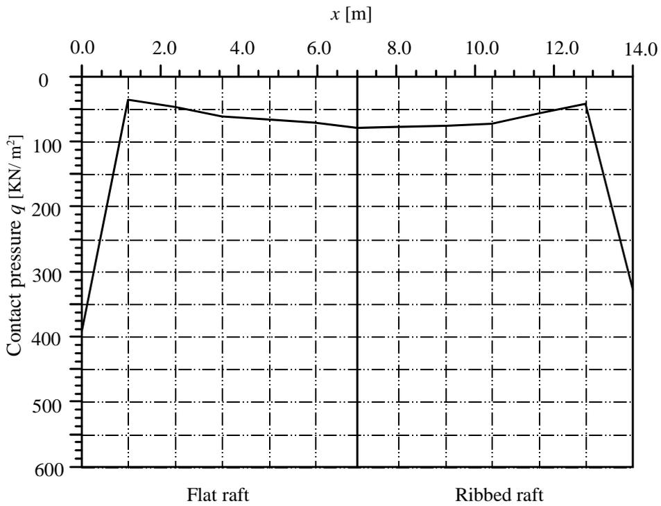
Figure 63 Contact pressures  $q$  [kN/m<sup>2</sup>] at middle section  $a-a$  for flat and ribbed rafts
