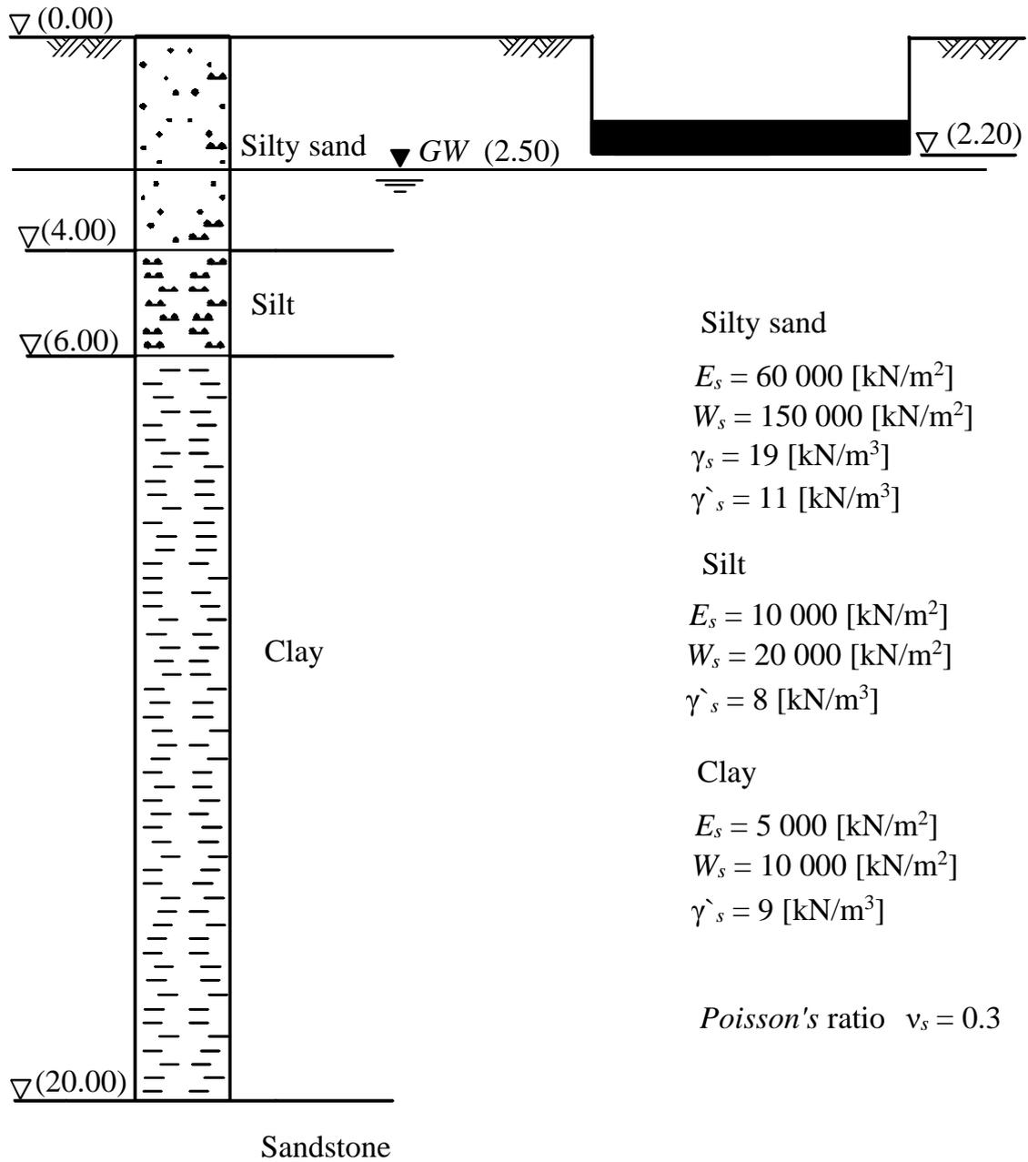
Figure 50 Soil layers and soil parameters under rafts
