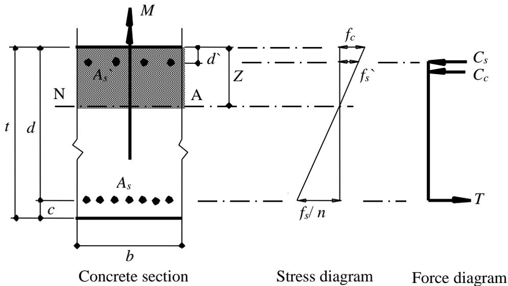
Figure 11 Distribution of stresses and forces according to ECP (working stress method)
