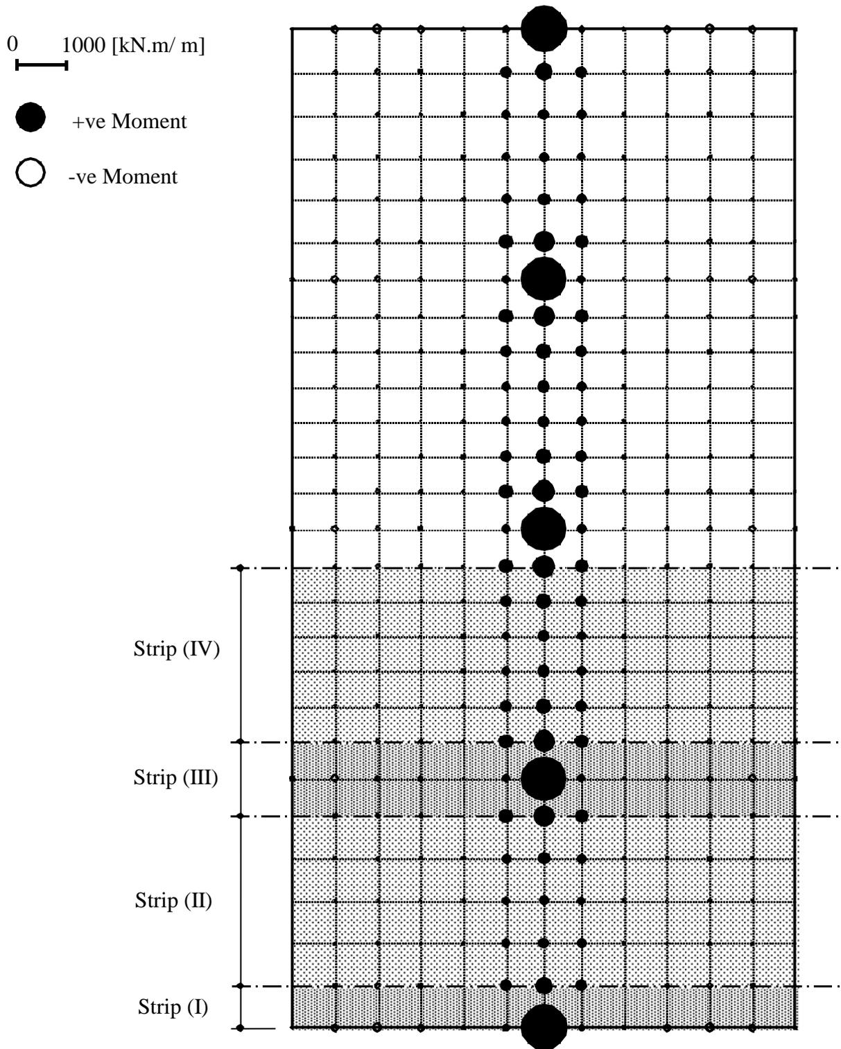
Figure 65 Circular diagrams of moments  $m_x$  [kN.m/ m] and critical strips in  $x$ -direction
