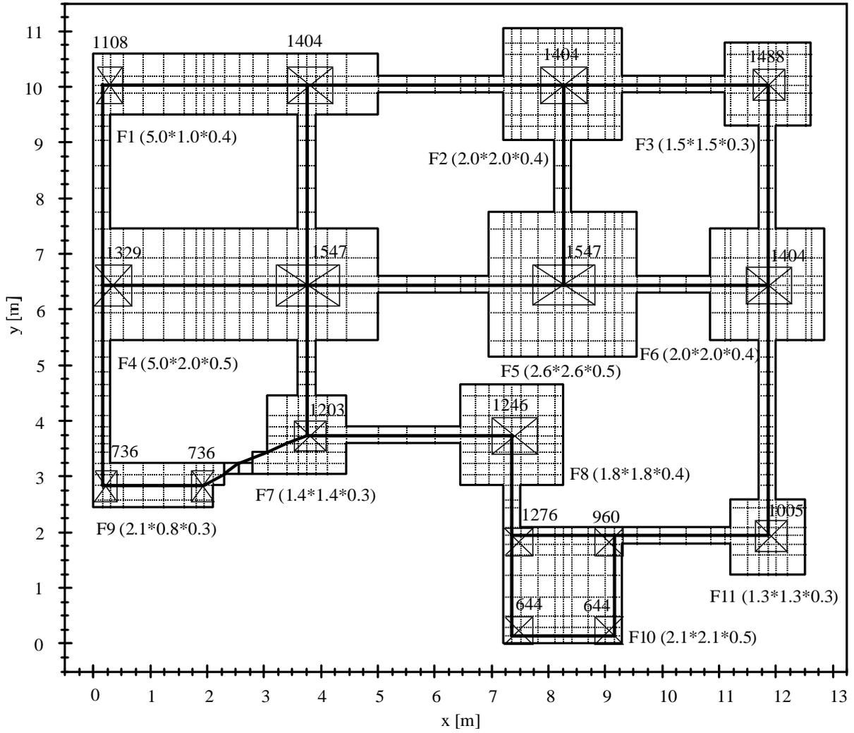
Figure 89 FE-Net of footings with tie beams, loads [kN/m<sup>2</sup>] and footing dimensions [m]
