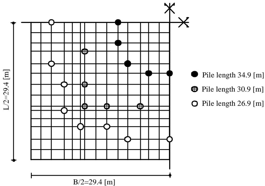
Figure 4-3 Mesh of *Messeturm* piled raft with piles (Max. element length = 2.0 [m])
