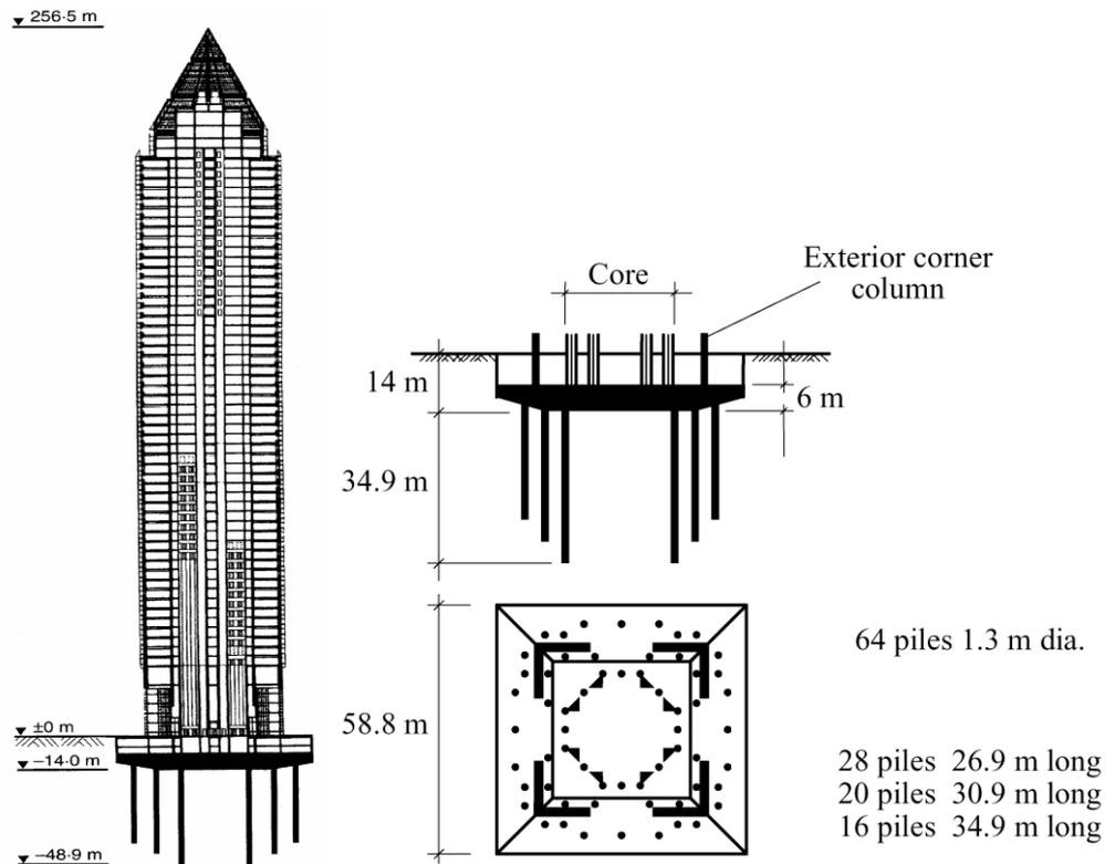
Figure 4-2 Layout of *Messeturm* with piled raft after *Chow/ Small* (2005)
