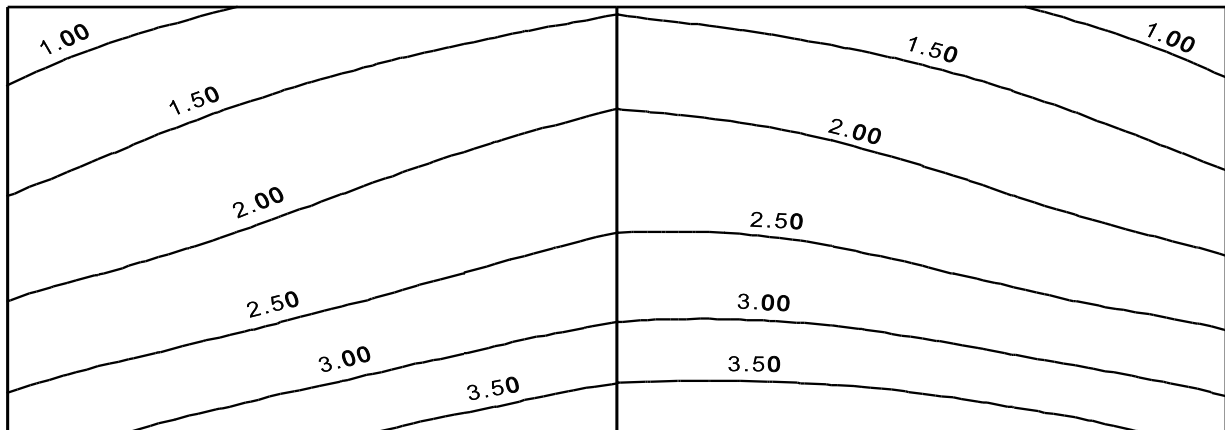
Figure 4.63 Contour lines of settlements s [cm] Analysis with interaction and with shearing forces (case 3) With influence of surrounding loading
