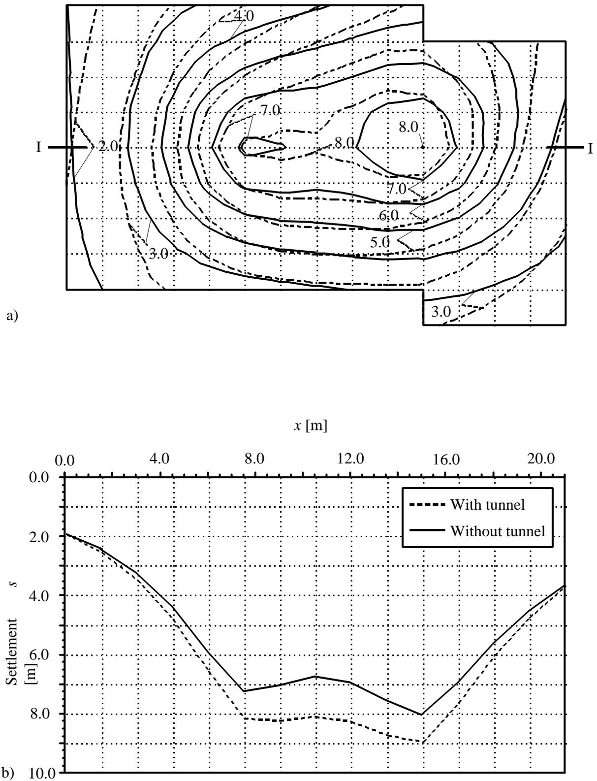
**Figure 3.11** Settlements  $s$  [cm] without and with consideration of the tunneling
