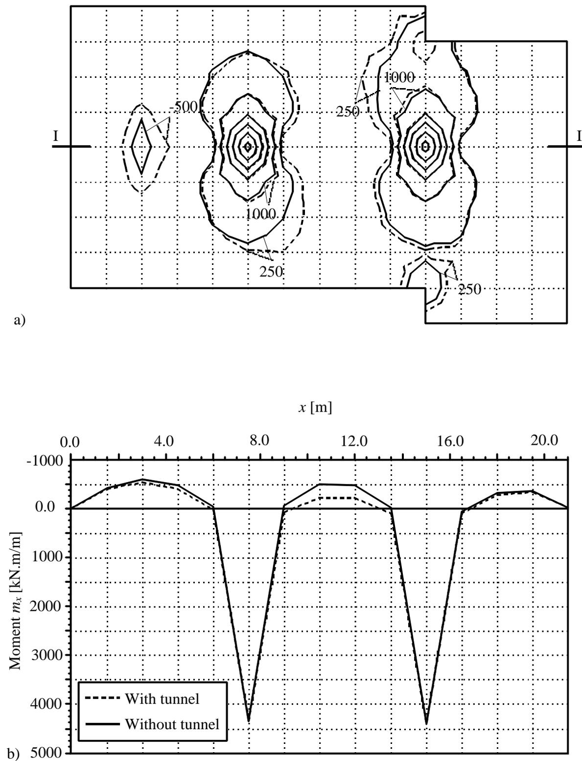
Figure 3.13 Moments  $m_x$  [kN.m/m] without and with consideration of the tunneling
