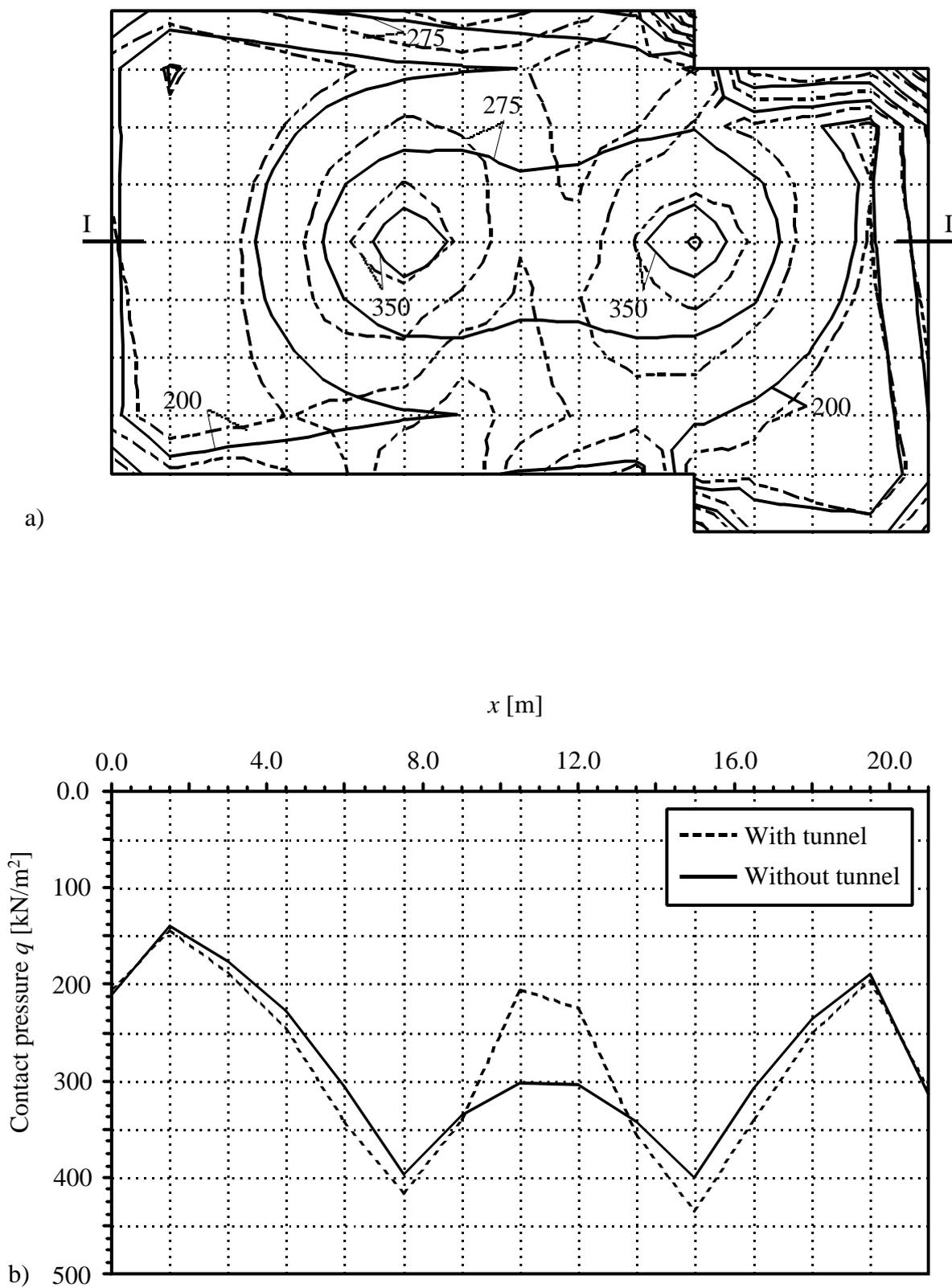
Figure 3.12 Contact pressures  $q$  [ $\text{kN/m}^2$ ] without and with consideration of the tunneling
