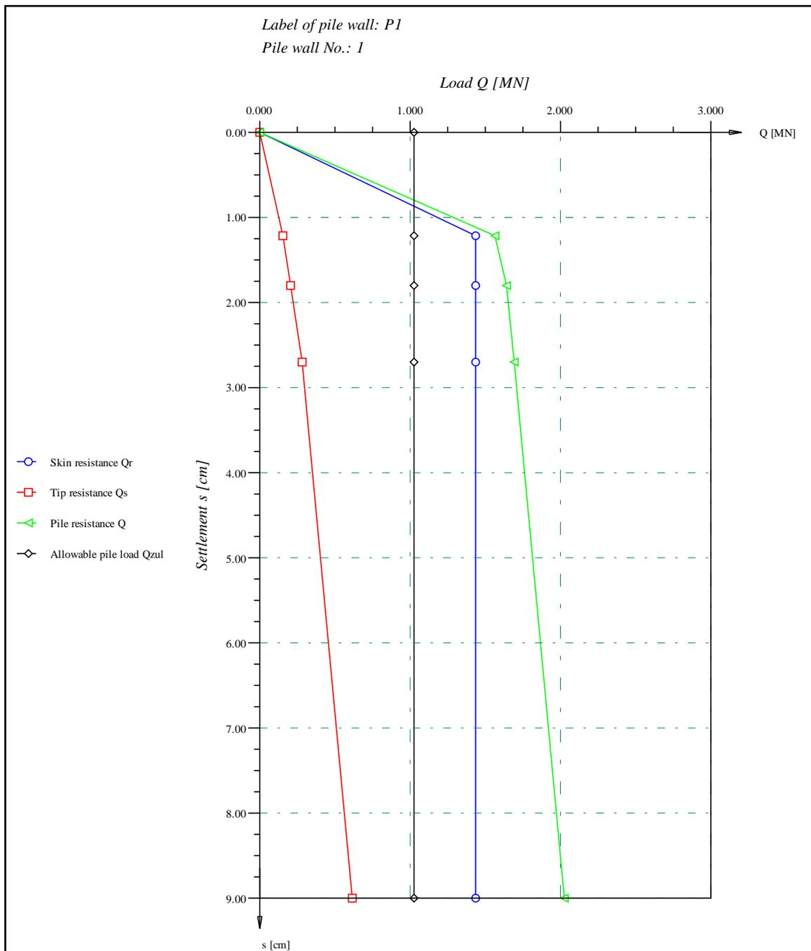
Load settlement curve of pile according to DIN 4014
