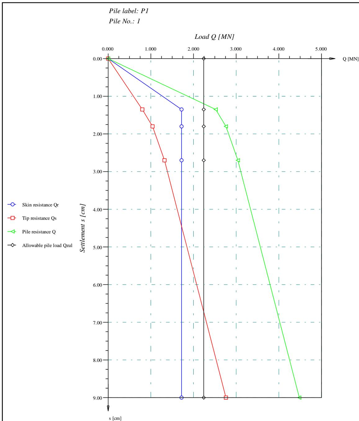
Load settlement curve of pile according to EA-Piles for upper table values
