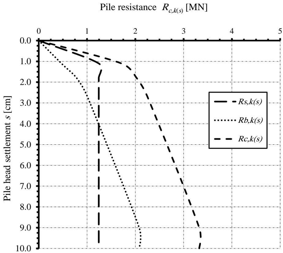
Figure 14 Resistance-settlement curve (lower values) "EA-Piles"
