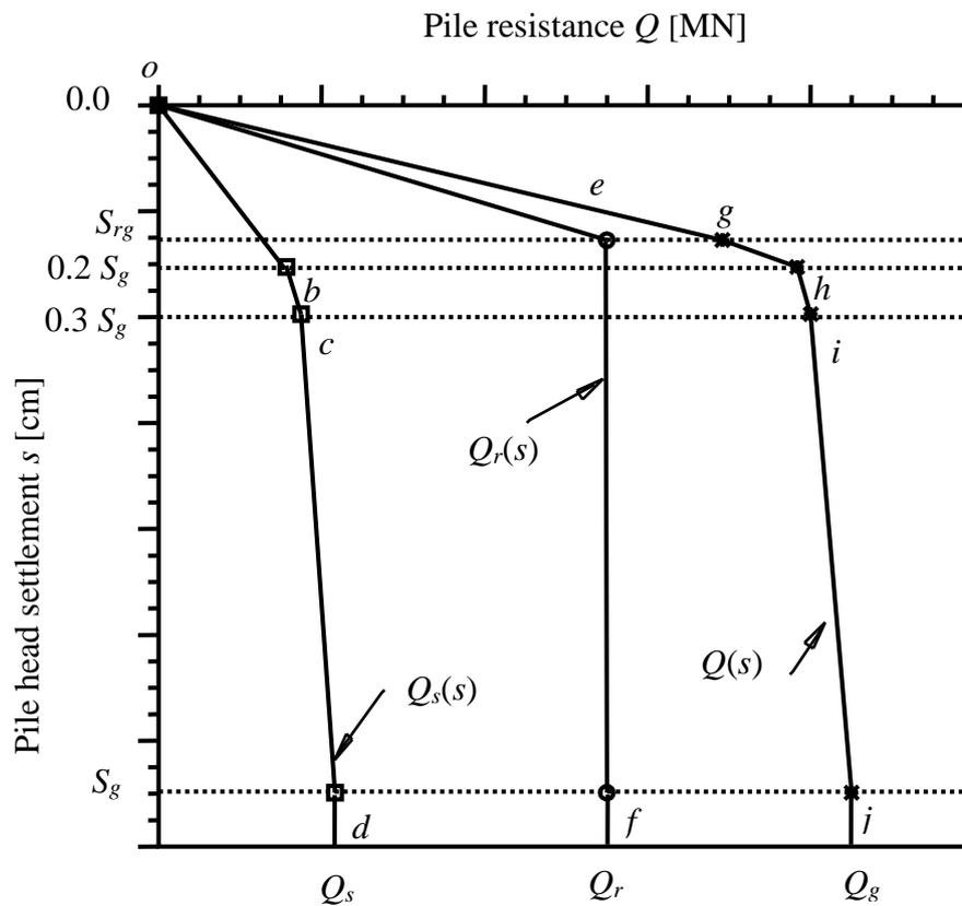
Figure 1 Construction of the resistance line using the tables 1 to 6
