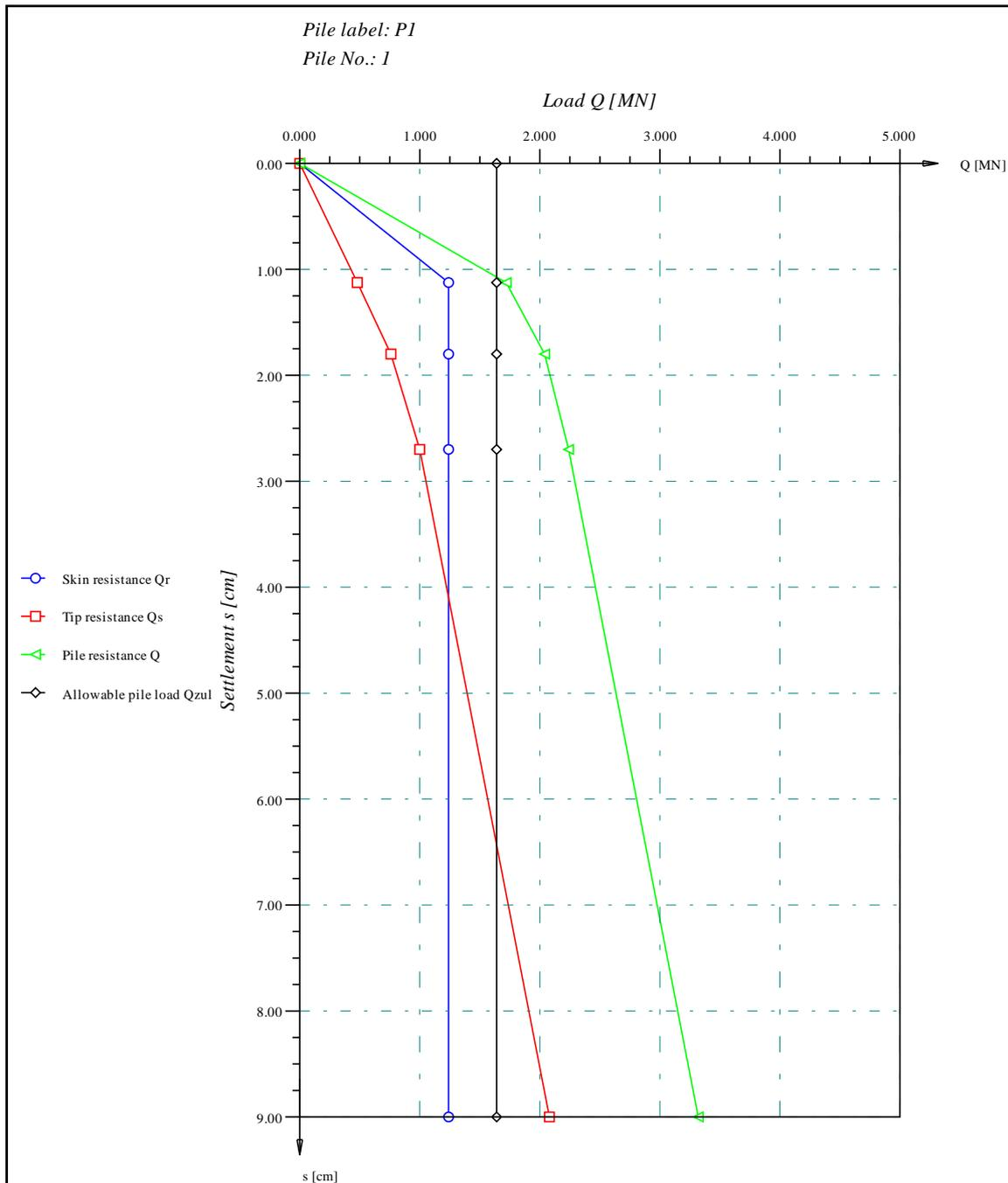
Load settlement curve of pile according to EA-Piles for lower table values
