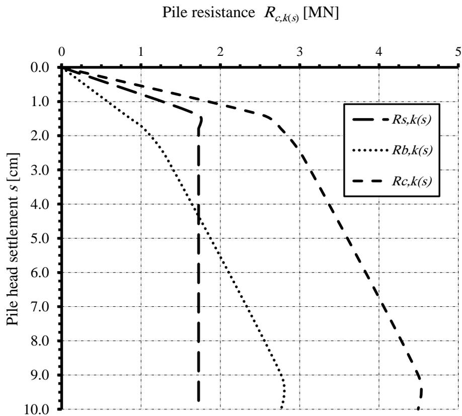
Figure 15 Resistance-settlement curve (upper values) "EA-Piles"
