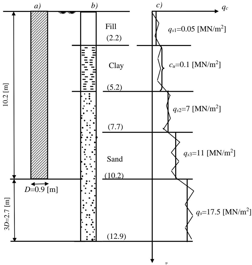
Figure 10 Soil profile, sounding graph and pile dimensions for determination of load-settlement curve
