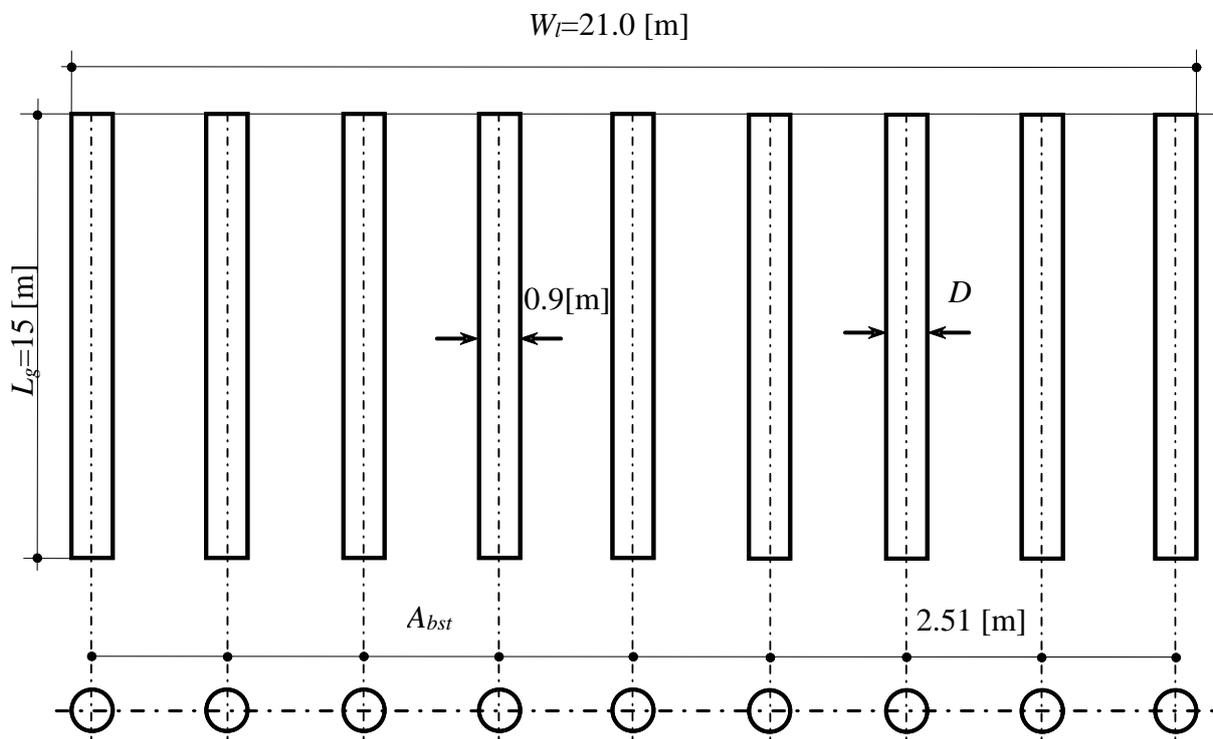
Figure 12 Dimension and data of the pile wall
