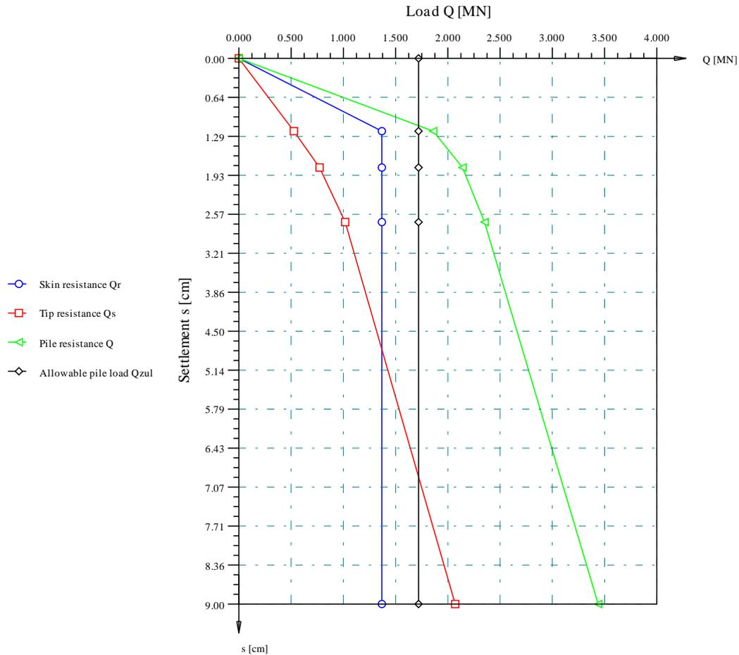
Load settlement curve of pile according to DIN4014
