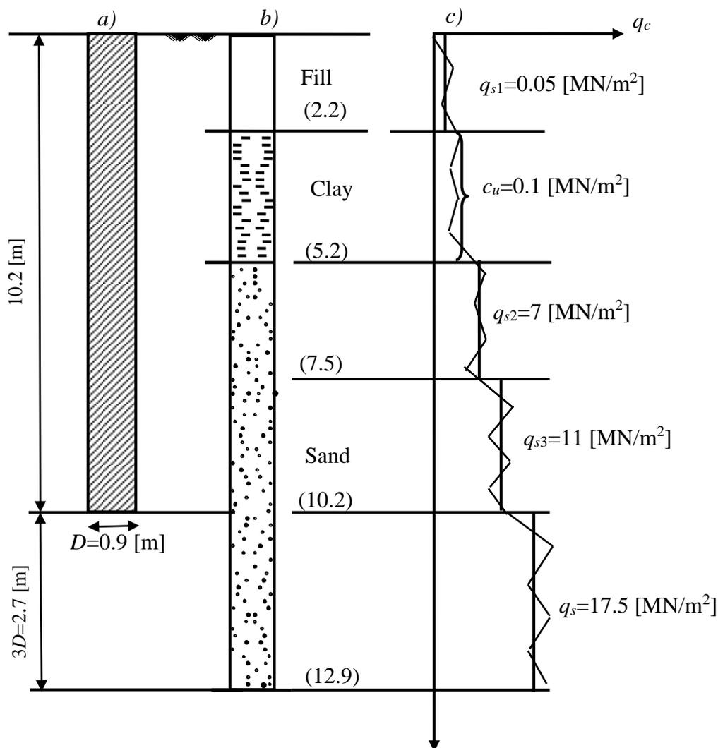
Figure 13 Soil profile, penetration test diagram and dimensions for an example calculation of the resistance-settlement curve;  $D=0,9$  [m],  $U=2,83$  [m],  $A=0,64$  [m<sup>2</sup>]
