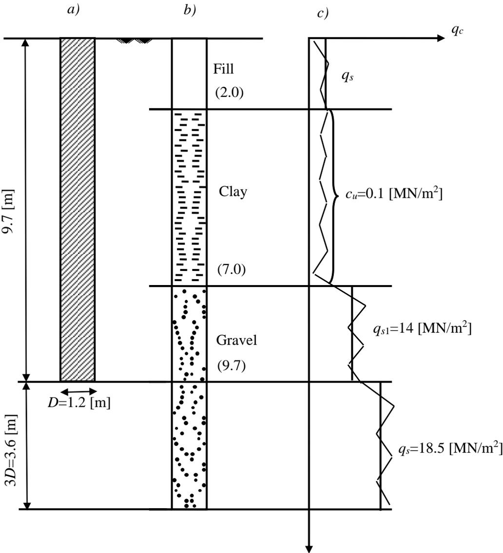
Figure 11 Soil profile, sounding graph and pile dimensions for determination of load-settlement curve
