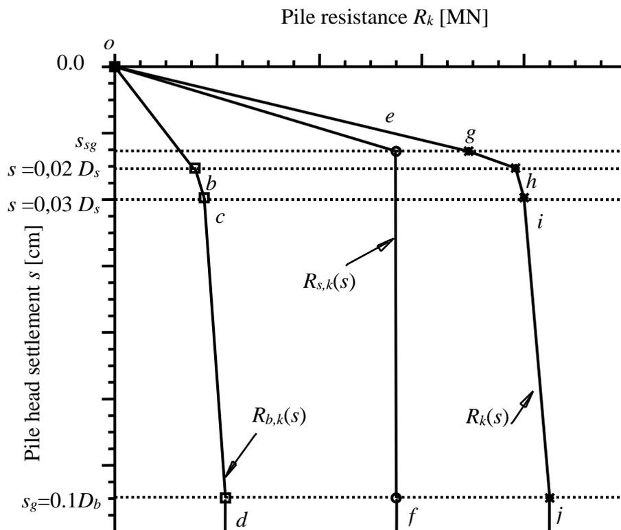
Figure 2 Elements of the characteristic resistance-settlement curve for bored piles
